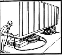
C. NEVER work under a load supported by only the air lifting bag.
