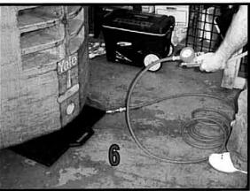
7. When operating the controller with (2) air lifting bags connected, practice operating the bags simultaneously and alternately, inflating and deflating. As you can see, the operation of the air bag system is simple.
