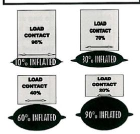
When only partial surface area of bags contact the load– lifting capacity varies in relation to load weight and bag arc.
