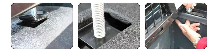
5. Slide the window guard over the right bracket now and install the 2 bolts and washers in the width adjusting slots, do not tighten just snug them up at this point.
