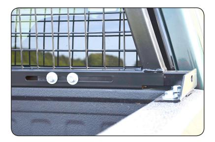
6. Slide the left bracket into the window guard and install the 2 bolts and washers, just snug them up.
