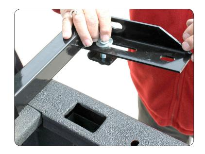
3. Note the mounting brackets use the stake pocket anchor holes for mounting.
