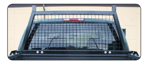
9. Now we need to drill a  $\frac{1}{2}$ " hole in the truck box to finish securing the left and right brackets, using the remaining 2 bolts and washers place them in the holes, using the remaining black flat brackets (with welded nut on the bottom) to tighten these into place.
