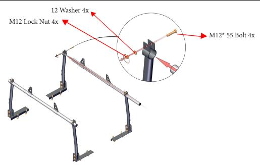
4. Place the assembled cross bar onto the opening tops of each post (3), tighten with M12\*55 Bolts" (19), 12 washers (6), and M12 Lock nuts (20).
