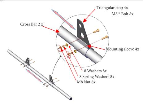
1. Slide 2 mounting sleeves (14) onto one of the cross bars (4). Insert the triangular stops(13) into the mounting sleeve(14), secure with M8\*25 Bolts(15) and 8 washers(16),8 spring washers(17),M8 nuts(18). Repeat for 4 triangular stops.
