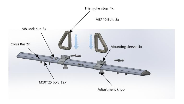
1. Slide triangular stop (3) into a mounting sleeve (4), tighten with M8\*40 bolt (5) and M8 lock nut (6). Repeat until all 4 triangular stops are assembled.
