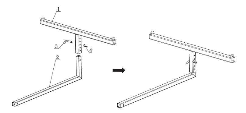
The extender can be assembled two different ways, respectively with the long end or short the end of L-extension (2) connecting to the T-support(1)
