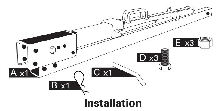
**Step 1** Insert the Big Bed (A) apparatus into a properly mounted hitch (not included) that has a **2 inch receiver**. Install hitch pin (not included) to secure the Big Bed.
