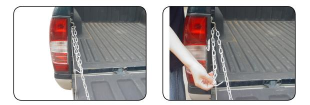
Step 3: Secure the ramp to the vehicle using the safety chain. After the safety chain is secure, test the ramp by pulling backwards on it. Make sure it does not slide back or disengage from the loading surface.
