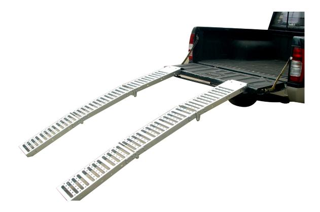
Step 2: Place the tongue of tri-fold ramp against the back of vehicle.
