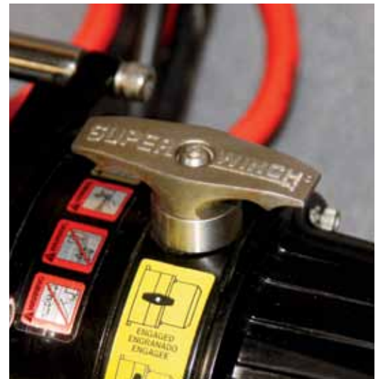
Our panel of judges gave mixed reviews on the unit's unique stainless steel T-handle clutch lever.
