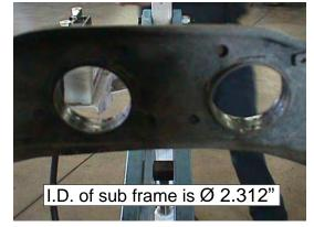
Remove O.E. outer metal shell, bushing and inner metal cup from sub frame.
