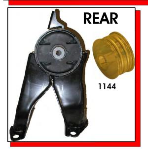
Press out factory shell and bushing in both positions.
