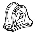
Clean any dirt, grease, and excess rubber flashing that may be present inside the engine mount. NOTE: IT IS VERY IMPORTANT THAT THE INSIDE OF THE ENGINE MOUNT BE CLEAN AND DRY.
