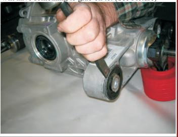
2. You will need to press the old bushings out. Using one of these process (See Picture Below)
