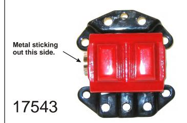
Assemble the two half together with the supplied nuts, bolts and washers. Install the bolts from the bottom with the washers and nuts on top. HINT: Due to the many different metal configurations from foreign and domestic manufacturers it maybe helpful to apply a thin coating of grease or dishwashing detergent to the polyurethane insert, at metal contact points before installing. This will allow the insert to seat, in turn allowing proper bolt alignment.
