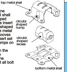
HINT: Due to the many different metal configurations from foreign and domestic manufacturers it maybe helpful to apply a thin coating of grease or dishwashing detergent to the polyurethane insert, at metal contact points before installing. This will allow the insert to seat, in turn allowing proper bolt alignment.
