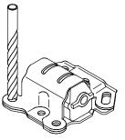
Clean any dirt and grease that may have accumulated inside the metal shells. NOTE: IT IS VERY IMPORTANT THAT THE INSIDE OF THE METAL SHELLS BE CLEAN. At this point, it is your option to have your metal painted, powder coated, or chromed.
