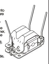
Make sure the tie-wraps are holding firm while releasing the clamp or vise. The metal shells may separate slightly, this is normal. However, excessive separation will prevent mounting botts from reaching through the crossmember allowing the nuts to start on the botts. Cut the ends of the tie-wraps off, being sure not to leave any sharp edges.
