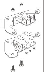
NOTE: The 3/8" bolts have a square on them which will "bite" on the inside of the 1/2" hole and keep them from turning. However, it may be necessary to use locking pliers to keep the bolt from turning while applying the proper torque.
