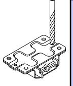
Clean any dirt and grease that may have accumulated inside the metal shells. NOTE: IT IS VERY IMPORTANT THAT THE INSIDE OF THE METAL SHELLS BE CLEAN. At this point, it is your option to have your metal painted, powder coated, or chromed.
