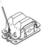
Make sure the tie-wraps are holding firm while releasing the clamp or vise. The metal shells may separate slightly, this is normal. However, excessive separation will cause the mounting bolts to not reach through the crossmember and allow the nuts to start on the bolts. Cut the ends of the tie-wraps off, being sure not to leave any sharp edges.
