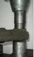
When pressing out bushings, it is good practice to remove and replace one at a time to maintain good rear alignment.
