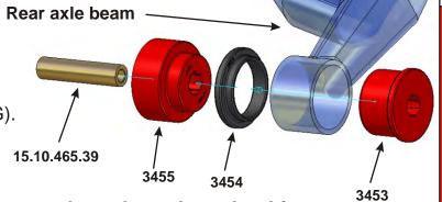
Apply grease to all metal parts that contact the polyurethane bushings.
