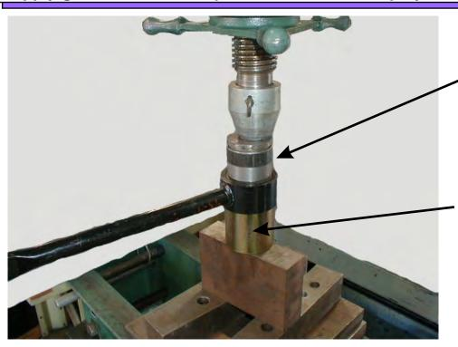
Inside Dia. of tension rod is 2.512" (63.8mm). Push out old bushing with something smaller than 2.512".
