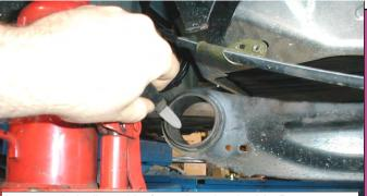
Let metal shell cool before cleaning inside Remove any burrs and sharp edges before applying grease. With both eyes of the trailing arm smooth, clean, and free from sharp metal burrs and any metal shavings.
