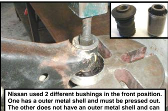
be pushed out with an arbor press. The I.D. of the O.E. control arm is Ø1.265" and is the same size for both.
