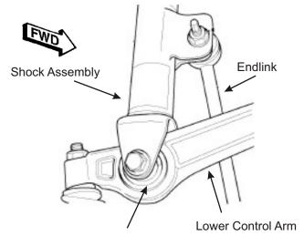
WARNING: DO NOT REMOVE SHOCK MOUNTING BUSHING FROM LOWER CONTROL ARM!!!! THIS BUSHING IS NOT & WILL NOT BE SUPPLIED OR A REPLACEMENT MADE FOR THIS POSITION!!!
