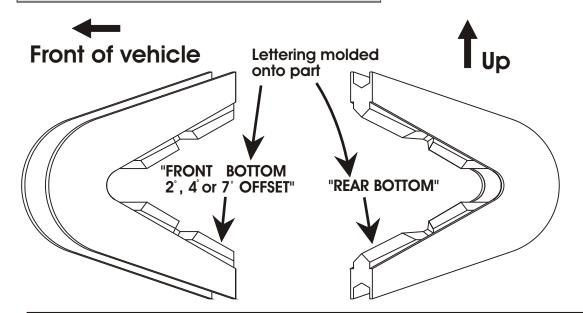
C-bushings are available in 2,4 and 7 degree positive caster. The recommended usage for the C-bushings is:
