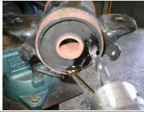
**Step 2:** Apply heat to the outer metal shell until the rubber bond is broken. When you see a good amount of white smoke then the bond should be broken. At no time should there be a flame from the rubber, if there is then back off the heat. Slide the entire outer shell off the inner sleeve. Do not damage the outer shell because it must be re-used with bushing 3473.
