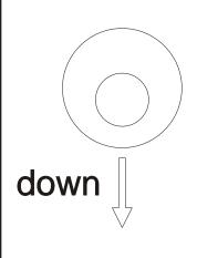
Bushings must be installed with offset hole down and centered in the 6 o'clock position.
