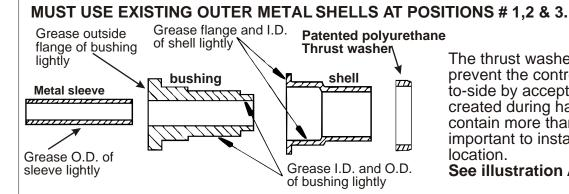
The thrust washers are designed to prevent the control arm from walking sideto-side by accepting side load pressure created during hard cornering. Most kits contain more than one part #. It is very important to install them at the correct location.
