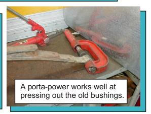
When installing Urethane bushings, apply grease as instructed: Remove the original rubber and outer shell (when used) clean I.D. of the spring eyes and frame brackets of any old rubber or rust with sand paper. Apply a light coat of grease to the eyes of both spring and frame brackets. Apply a light coat to the I.D., O.D. and flange of the bushings. (all surfaces that contact metal) Apply a light coat of grease to the O.D. of the sleeves.)
