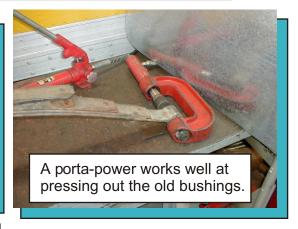
When installing Urethane bushings, apply grease as instructed: Remove the original rubber and outer shell (when used) clean I.D. of the spring eyes and frame brackets of any old rubber or rust with sand paper. Apply a light coat of grease to the eyes of both spring and frame brackets. Apply a light coat to the I.D., O.D. and flange of the bushings. (all surfaces that contact metal) Apply a light coat of grease to the O.D. of the sleeves.)
