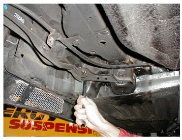
**Step 1.** Remove <u>outer</u> compensator arm <u>bolt only</u>. Remove two mounting bolts at cross pin, and parking brake cable retainer. At this time it is your discretion to remove complete trailing arm from vehicle to facilitate easier removal and installation of new polyurethane bushing or you may pull front of trailing arm downward.
