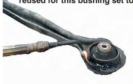
Apply light heat evenly around the outside of the outer metal shell, just enough to brake the bond with the rubber. When you see light smoke coming from the sides of the bushing the bond should be broken. At no time should there be any flames coming from the rubber, if there are any flames, you need to back off with the heat. Just push the old rubber and inner metal sleeve out. Let the outer metal shell cool before cleaning the inside.
