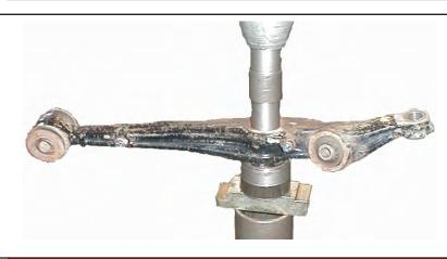
A hydraulic press was used to remove the original bushing, including the outer metal casing the rubber is bonded to. The inside diameter of the control arm is Ø 36mm (1.417"). Go about .050" smaller when pressing out the bushing.
