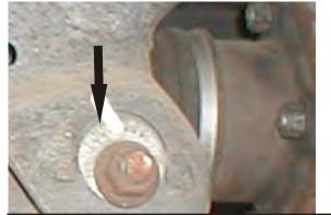
Remove the stock bushings from both control arms using heat rather than a hydraulic press to avoid accidentally bending the control arms.
