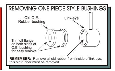
NOTE: All 4 control arms (2 upper 2 lower) use the same bushing for all 8 positions. Factory rubber bushings are not bonded.
