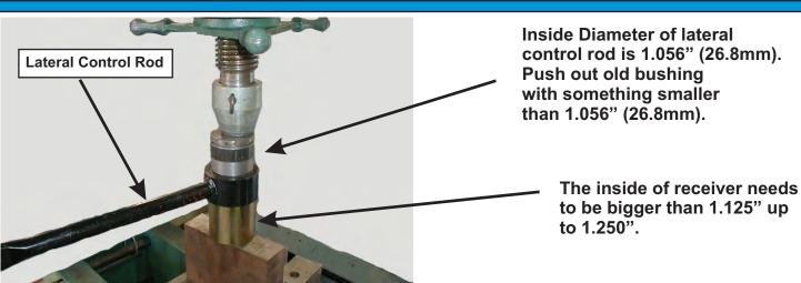
The old rubber bushing is not bonded to the eye. When pressing out the original bushing, you need to push it with something smaller than the inside diameter of the lateral control rod. And the receiver end needs to be bigger than the outside diameter of the old bushing being pushed out.
