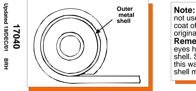
**Note:** When a sleeve is not used, apply a light coat of grease to the original shoulder bolt. **Remember:** Most spring eyes have an outer metal shell. Some shackles are this way as well. The outer shell must be removed.
