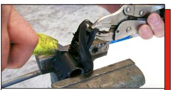
Inner sleeve is bonded with the old rubber bushing. To remove the old rubber bushing from the sleeve, clamp the sleeve in a vice and using a utility knife, slice the bushing longways away from yourself. Clamp the bushing with vicegrips pulling the rubber back and slice as close to the sleeve as possible. Rotate the sleeve in the vice until you get all the way around. Clean as much rubber off the sleeve until smooth.
