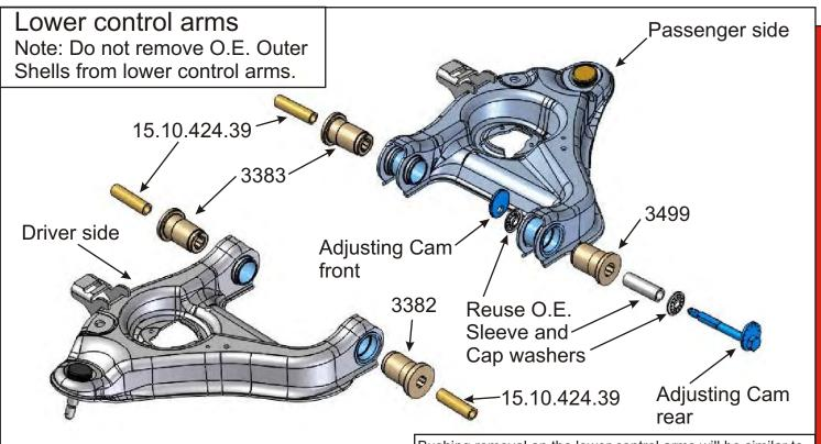
Be sure to place matchmarks on the front and rear of the adjusting cam before you start. You will need to use these matchmarks to reinstall the passenger side lower control arm back in the same position after the new polyurethane bushings are installed. Then have the vehicle's alignment checked by a certified technician . The alignment must be within factory specifications.
