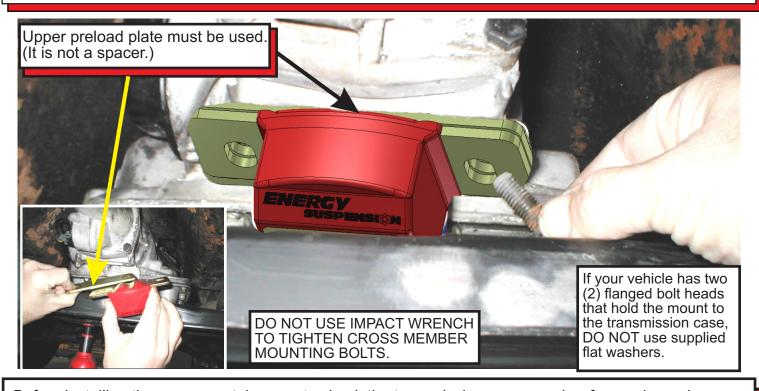
Before installing the new mount, be sure to check the transmission crossmember for cracks or damage at the slotted hole areas. Repair or replace the crossmember if any damage is evident. On high performance(race condition) applications, reinforcing the area around the mounting point of the crossmember is recommended. This type of crossmember has an inherent problem with stress cracks around the bolt holes. Always check the front engine mounts and replace if necessary.
