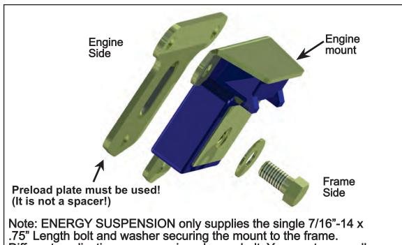
Different applications may require a longer bolt. You must reuse all bolts securing the mount to the engine block.
