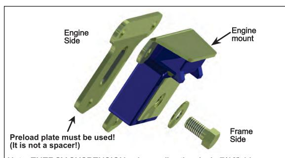
Note: ENERGY SUSPENSION only supplies the single 7/16"-14 x .75" Length bolt and washer securing the mount to the frame. Different applications may require a longer bolt. You must reuse all bolts securing the mount to the engine block.
