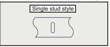
Before installing the new mount, be sure to check the transmission crossmember for cracks or damage at the slotted hole areas. Repair or replace the crossmember if any damage is evident. On high performance(race condition) applications, reinforcing the area around the mounting point of the crossmember is recommended. This type of crossmember has an inherent problem with stress cracks around the bolt holes. Always check the front engine mounts and replace if necessary.
