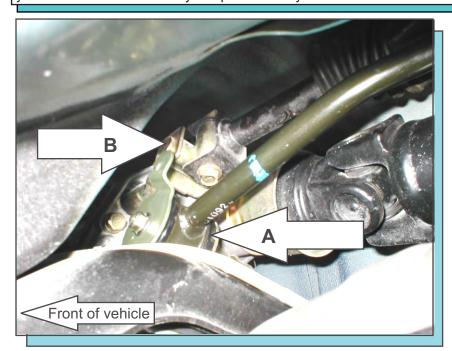
**Note:** Do not remove the upper shifter linkage (See arrow B).
