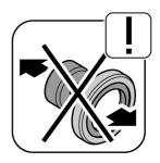
• Before assembly of the oil seal, the shaft surface must be carefully inspected to ascertain that it is free of grooves or other damages. If this is not the case, these must be removed. If in doubt, it is absolutely necessary to consult an engine specialist/repairer who will possibly perform a professional surface finishing, if needed.
