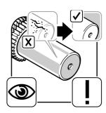
Important: The PTFE oil seal must be installed dry. Oil or grease of any kind must NOT be used as an assembly agent.
