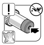
For assembly, the plastic cover is positioned such that the oil seal can smoothly slide onto the shaft. An appropriate insertion tool must be used when sliding or pressing the oil seal onto the shaft, and it must be ensured that this occurs evenly and without impact load. Otherwise there is a risk of damaging the sealing lip, and flawless sealing function is no longer guaranteed.
