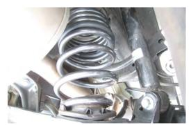
**Note:** PRO-KIT spring rates are measured as a system of the front or rear suspension. 10mm of bump-stop deflection is included in the final rate of the system. Lowering numbers based on coupe model. PRO-KIT will require alignment kit 5.67470K to align camber to OE specs
