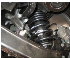
Note: PRO-KIT spring rates are measured as a system of the front or rear suspension. 10mm of bump-stop deflection is included in the final rate of the system.
