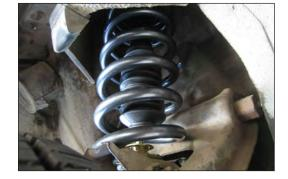
PRO-KIT spring rates are measured as a system of front or rear suspension. 10mm of bump-stop deflection is included in the final rate of the system.
