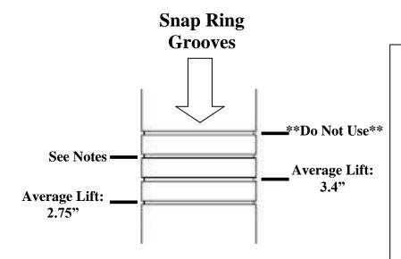
Important: Ensure that the snap ring is fully seated in the snap ring groove (you should be able to rotate the snap ring manually/by hand). Note: Improper installation will cause permanent damage to the shock. Please refer to the Pro Truck Sport Damper instructions for more info regarding proper installation and fitment.
