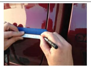
**STEP 2:** Position the Body Side Moldings onto the door to ensure an equal distance from rear back edge and front forward edge of the door, when aligned mark position with a non-permanent marker on masking tape. Ensure the correct Body Side Moldings are identified prior to installing to doors. Parts are identified on the back side of Body Side Moldings. (Left Hand Side shown above)
