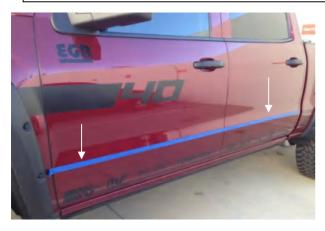
**STEP 1:** Ensure the door areas are clean and dry in the areas where the Body Side Moldings will make contact with the door surface. Apply masking tape to front and rear doors at desired height, if a ridge line is in the door profile ensure masking tape is applied to the top edge on ridge line. Ensure the masking tape is in a straight line to assist with aligning the Body Side Moldings to the front and rear doors.
