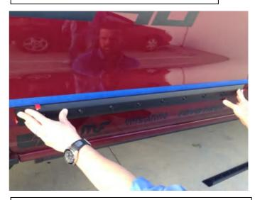
**STEP 4:** Aligning the rear end of Body Side Moldings with the position noted in step 2. Ensure the tape liners are facing outwards and apply light pressure in the exposed tape areas. If a ridge line is in door profile, position the Body Side Molding so the top edge of part runs below and parallel with the ridge line profile. (Left Hand Front shown above)
