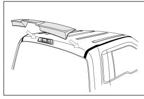
**STEP 1:** Test fit part on vehicle prior to install. Clean the areas on the roof where the cab spoiler will contact the sheet metal using soap and water. A secondary cleaning of isopropyl alcohol can be used, but is not required.
