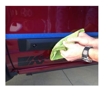
**STEP 6:** Using a clean, soft cloth, firmly rub down over the attachment areas to ensure maximum adhesion. Ensure top, bottom and ends of Body Side Moldings are rubbed down approximately 5 times using firm pressure. Ensure no gapping is evident along top, bottom and ends of Body Side Moldings.
