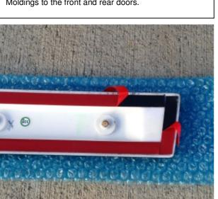
**STEP 3:** Peel back approximately 2" inches of protective tape liner, at alternating corners of the Body Side Molding, and fold to the outside at a 45 degree angle.
