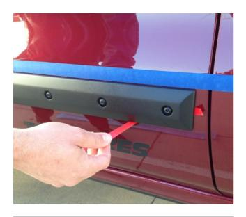
**STEP 5:** Ensure Body Side Molding is positioned correctly on the door surface in the desired location. Slowly peel the remaining tape liner away by pulling on the exposed ends of liner and apply firm pressure around the attachment areas.
