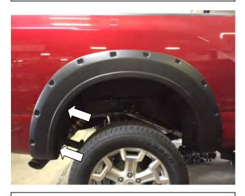
**STEP 11:** Place Fender Flare on the vehicle into the position of best fit. Note where (2) slots in rear of Fender Flare correspond with existing screws / fixing points in the wheel arch. Remove Fender Flare. Remove any existing vehicle screws in locations as shown with #2 Phillips head screwdriver. Maintain screws for re-installation.
